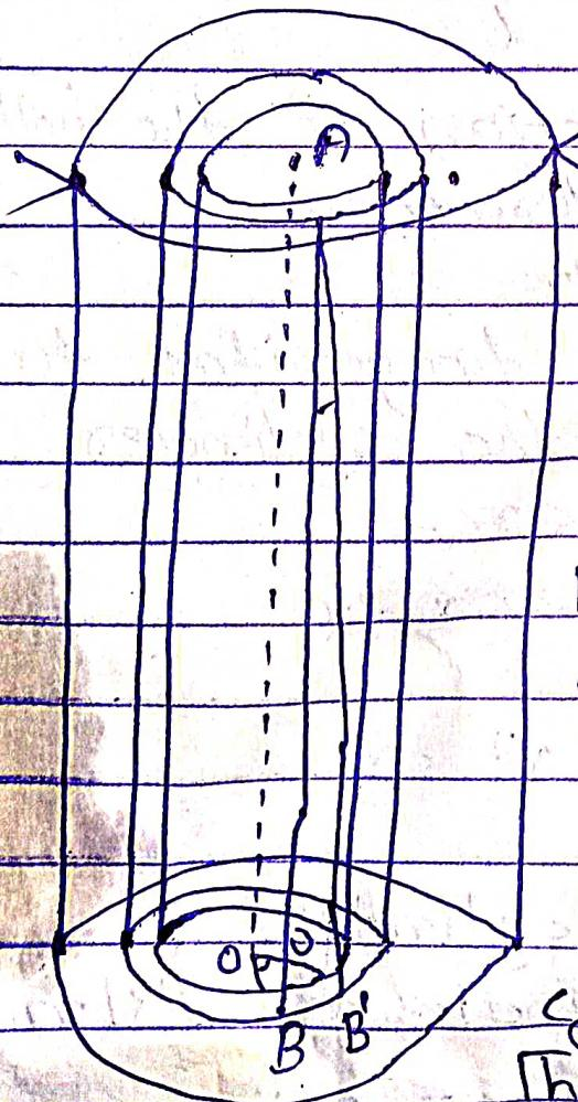
not change because it is a point on the clamped end. Then  $\angle BOB' = \theta$  will be called the angle of twist. Hence the angle of twist is the angle through which a radius of the free end is turned.  $\angle BAB' = \phi$  is the shearing strain at the surface of the hollow cylinder. Where as  $\theta$  is the same for all the hollow cylinders,  $\phi$  changes from cylinder to cylinder it is being
